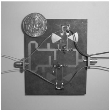
Fig. 2 Photograph of the new double-branch frequency doubler
