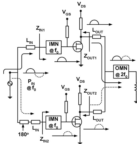
Fig. 1 Circuit diagram of the new frequency doubler (IMN@ $f_0$  and OMN@ $2f_0$  are input and output matching networks designed at fundamental and the second harmonic frequencies, respectively)
