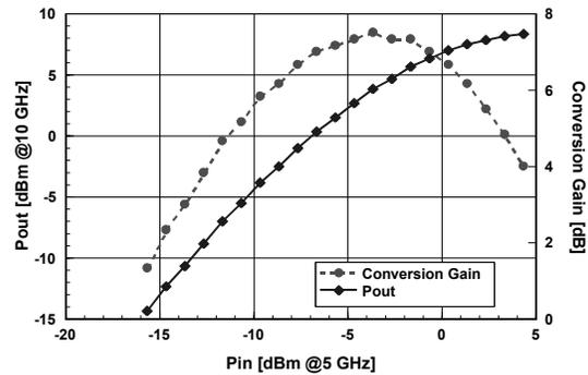
Fig. 3 Measured output power ( $P_{out}$ ) and conversion gain for the single-ended frequency doubler
