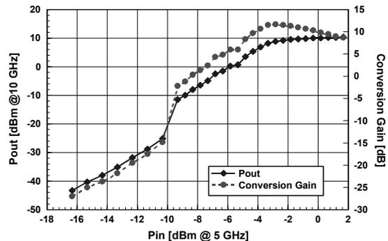
Fig. 4 Measured output power ( $P_{out}$ ) and conversion gain for the double-branch frequency doubler
