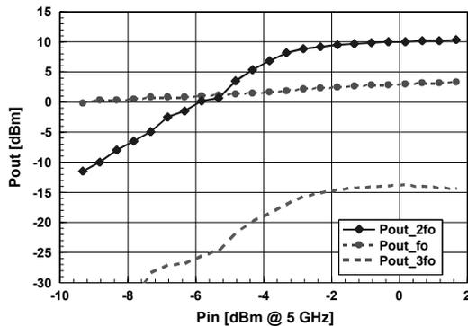
Fig. 5 Measured suppression characteristics of the double-branch frequency doubler
