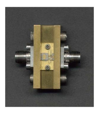
Fig. 2 Photograph of the AlGaN/GaN feedback power amplifier module
