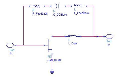
Fig. 1 Schematic of a shunt feedback amplifier with  $L_{\text{D}}$  and  $L_{\text{FB}}$
