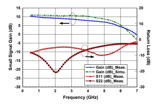
Fig. 3 Measured and simulated small signal characteristics of the amplifier
