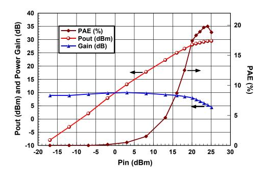
Fig. 4 Measured power characteristics of the amplifier
