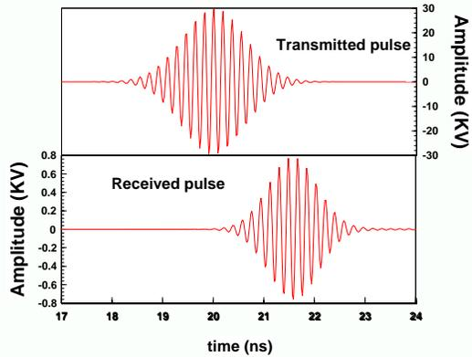
Gaussian Pulse Pulse width : 4ns
